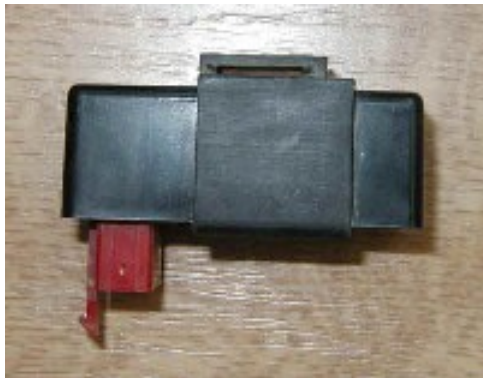
Pic 15. The original relay controlled by the electronics...
