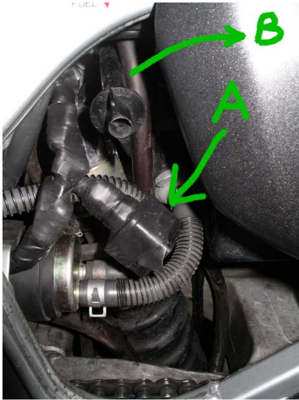
Pic 17. My relay location, A and better yet behind the cover, B.
